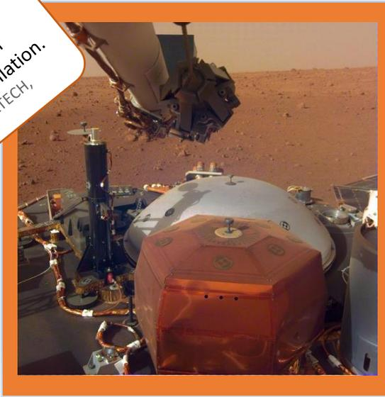
Photo of SEIS after its deposit on the martian surface
